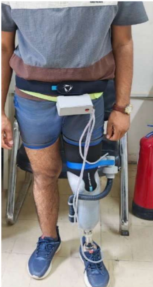
Fig. 9. Experimental setup showing the transtibial amputee participant fitted with the smart vacuum-assisted suspension system.
