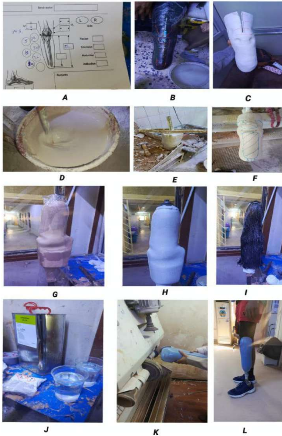
Fig. 1. Fabrication process of a transtibial (below-the-knee) prosthetic socket.
