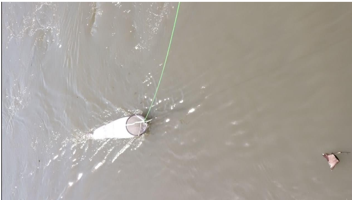
Fig. 2 Planktonic net used in the sampling process.
