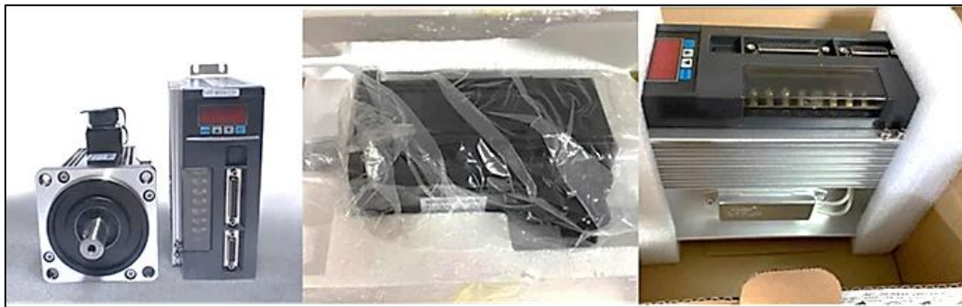
Figure 2: (2000W) Servo drive system
