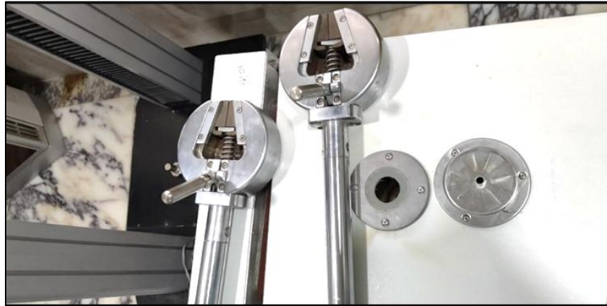
Figure 4: Modified grips capable of providing up to 50 kN gripping force.
