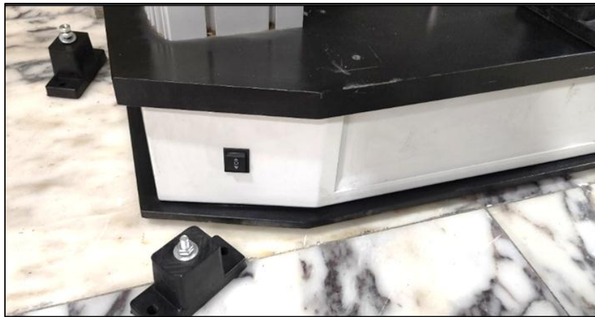
Figure 5: Custom-engineered rubberized vibration-dampening mounts
