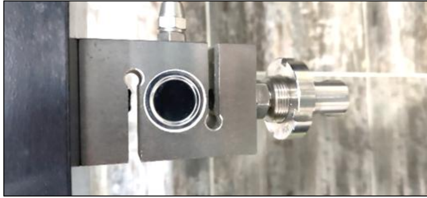
Figure 3: The upgraded and modified 50 kN load cell
