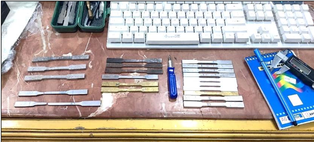
Figure 1: A group of tensile specimens was prepared and tested according to the ASTM standard
