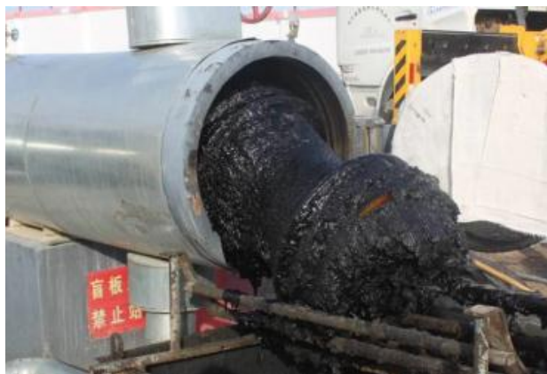
Figure 1: Wax Deposition in pipelines.
