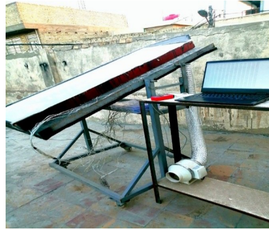
Figure 1. Experimental setup of the solar air heater (SAH) in this research
