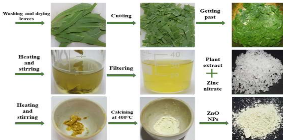
Figure 1: Green synthesis and characterization of zinc oxide nanoparticles using Eucalyptus . Leaf extract and zinc nitrate hexahydrate salt (12).
