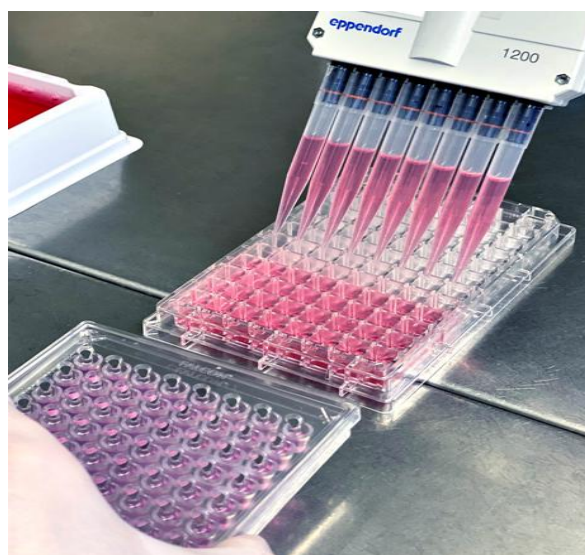
Figure 1: Preparation of 96-well microplate by multichannel pipetting of gold nanoparticle dilutions for MTT cytotoxicity assay against MCF-7 and MDA-MB-231 cancer cell lines.
