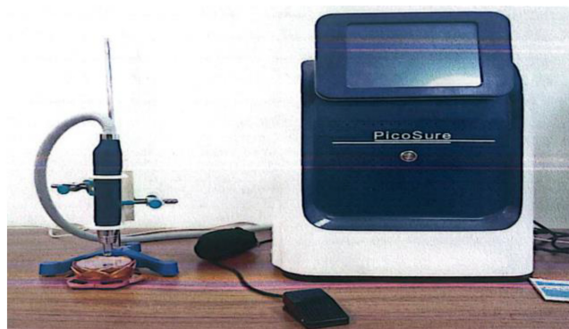
Fig. 1. A photograph of the pulsed laser ablation system.
