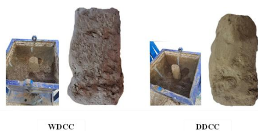
Fig. 9 Images showing the densification of the soil-cement columns
