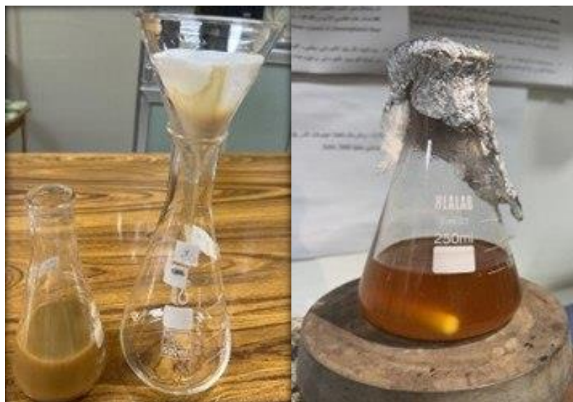
Figure1 : Steps and color profile change of the aqueous extract of Anastatica hierochuntica after addition of gold chloride
