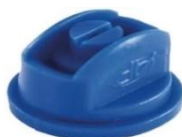
Figure 1. The APS80R 03C nozzle, which operates at an 80° spray angle and a recommended pressure range of 3–20 bar. This nozzle is ideal for applying fungicides and insecticides due to its effective droplet distribution and coverage. ( https://agroplast.pl/en_US/i/About/29 )
