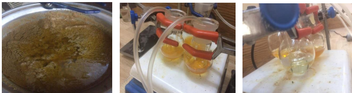
Figure 1- The Result of the Mechanical Digestion of the Fish Guts before and after Heating.
