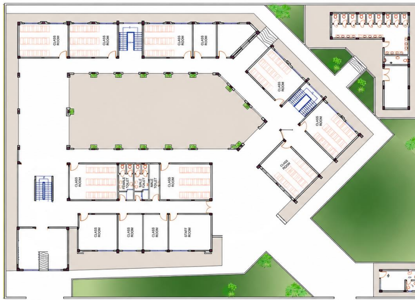
Figure (4): Ground-floor plan of the B18 model. Source: School Buildings Division, Al-Karkh First Directorate of Education [18].
