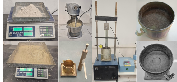
Figure 3. Application stages of the CBR test.
