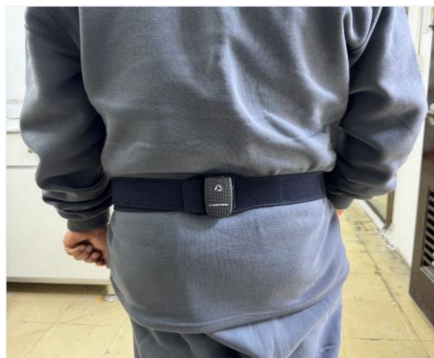
Fig. 2. Placement of the BTS G-Sensor at the level of the fifth lumbar vertebra (L5) using an elastic belt during gait data acquisition.
