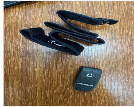
Fig. 3. BTS G-Sensor (G-Walk system) inertial measurement unit (IMU) and elastic mounting belt used for spatiotemporal gait analysis.
