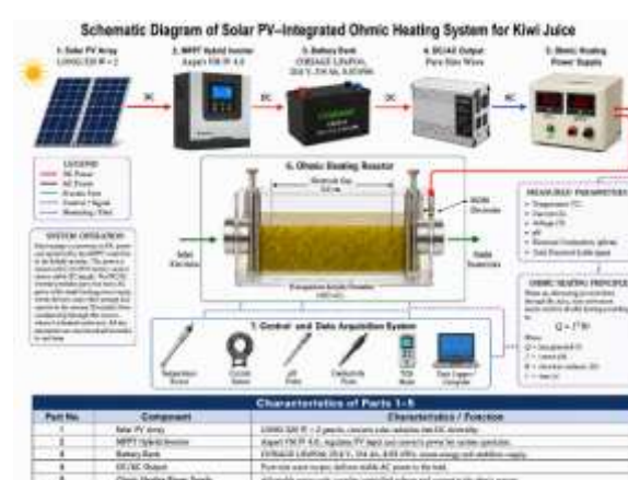
Figure 1. Schematic diagram of the solar PV-integrated ohmic heating system used for kiwi juice pasteurization.
