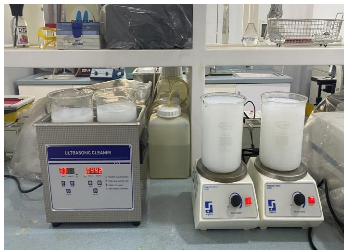
Figure 5: Magnetic stirrer and ultrasonic homogenizer (Hassan, Yaqob and Abdullah, 2023)
