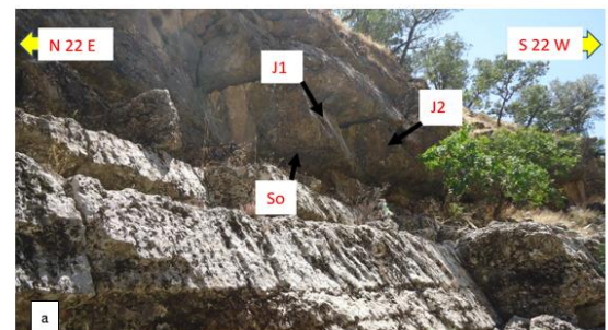
Figure 10: a- Field image with distinct discontinuity sets for station no 7. b- Planar sliding on the J1 is seen in kinematic analysis for station no.7. c- Wedge sliding on (J1 & J2) is seen in kinematic analysis for station no. 7. d- Flexural toppling about So is seen in kinematic analysis for station no. 7.
