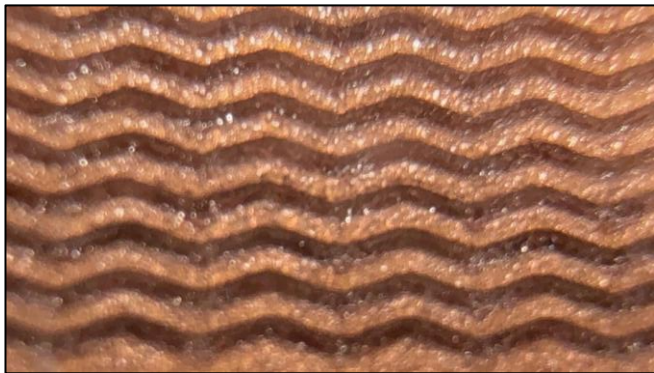
Fig. 17 Small scattered bubbles at a temperature of 180 \text{ kW/m}^2 .
