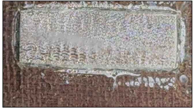
Fig. 19 There is a significant loss of liquid film with almost complete drying at heat fluxes of 780 \text{ kW/m}^2 .
