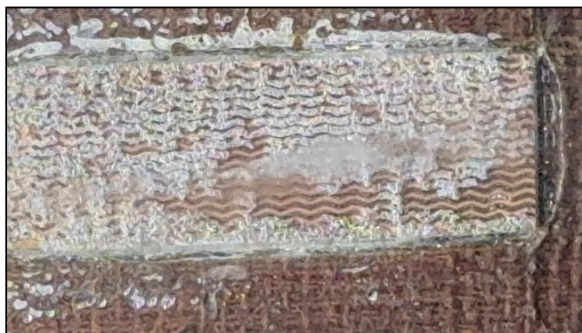
Fig. 18 Clear irregular annular flow at heat fluxes 500 \text{ kW/m}^2 .
