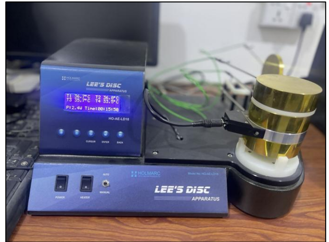
Fig. 3 The laboratory setup of Lee's apparatus.
