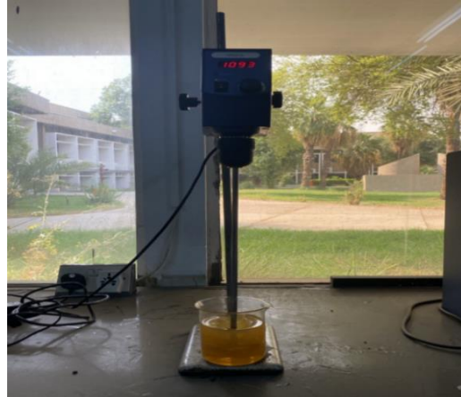
Fig. 2. Dispersion of NPs into lubricating oil by an electrical high-speed homogenizer
