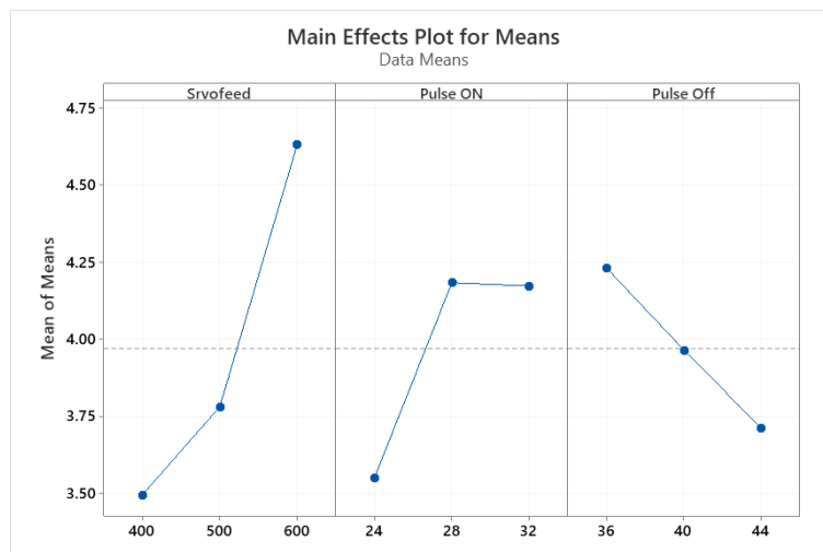
Fig. 3. Main effect plot for means of Ra
