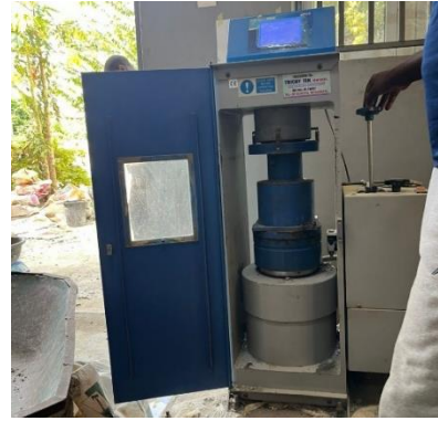
Fig. 2b. aggregates crushing value test
