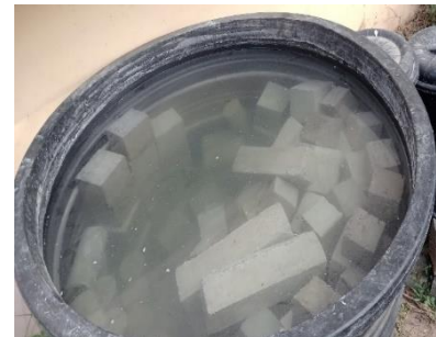
fig. 1c. Concrete samples incorporating steel slag
