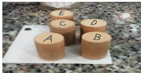
Fig. 1 Schematic representation of tested specimens. The samples in this study: sample A (W0), sample B (W10), sample C (W20), sample D (W30), sample E (W40).
