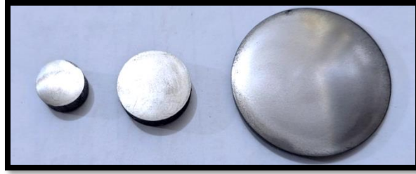
Fig. 1 shows the shape of the samples after the Grinding process Final samples were manufactured according to different gallium percentages as shown in Table7 .
