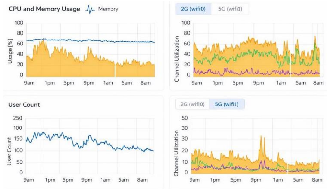
Fig. 12. Statistics on UniFi device connections for the 2G and 5G bands, including usage percentage, channel utilization, and number of users.
