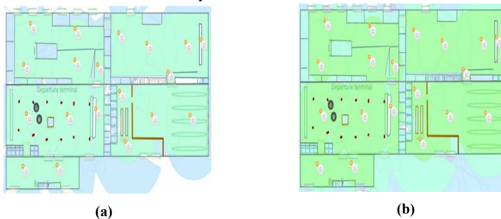
Fig. 7. The coverage rate in the passenger terminals using the UniFi Lite device at a height of 8 meters is measured when the received power is -65 dBm and -70 dBm.
