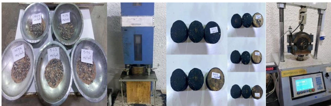
Fig. 1. Marshall specimen preparation and testing process
