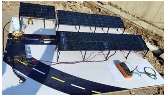
Fig. 10. Prototype model feed lamp load (18W)
