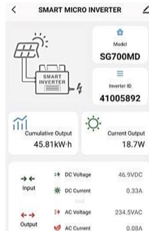
Fig. 14. Data from smart inverter at irradiance 760\text{W/m}^2
