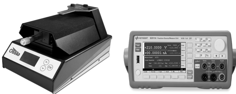
Figure 3.1. Electrical conductivity measurement setup used for I–V characterization of nano-doped organic semiconductor thin films.
