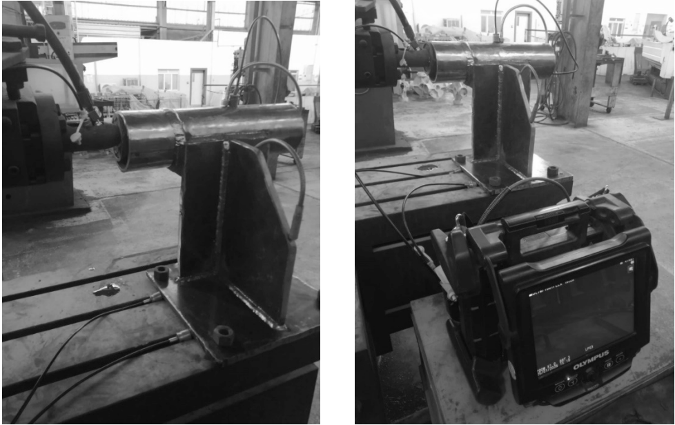
Figure 5 - Experimental setup showing the mounted bracket–pipe specimen installed on the vibration test rig, including the electrodynamic shaker, loading rod, rigid support frame, and boundary condition configuration used for dynamic excitation.
