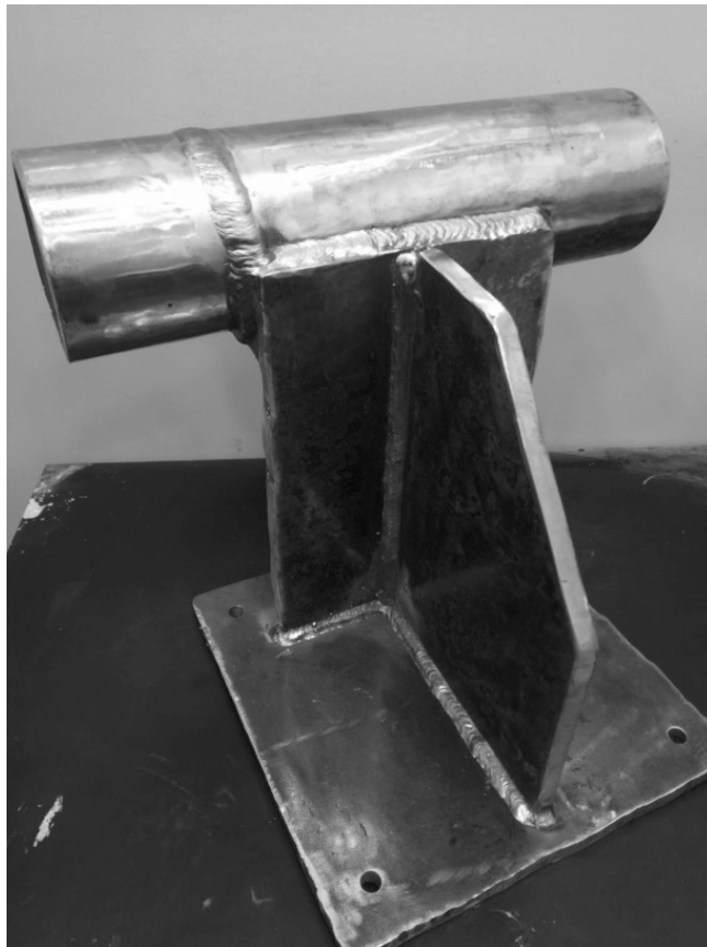
Figure 4 – Welded bracket–pipe specimen fabricated for the experimental program using Shielded Metal Arc Welding (SMAW) with E7018 low-hydrogen electrodes. The photograph shows the welded joints at the bracket–arm and bracket–base connections prior to instrumentation and testing.
