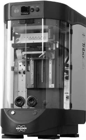
Figure 2. Bruker UMT TriboLab, a type of advanced tribometer used in Iraqi university research labs for friction and wear analysis.
